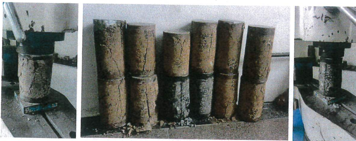
Photo 18 Failure pattern of UCS test cubes
