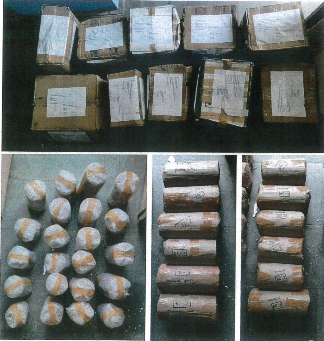
Photo15 Packing of field cores for transportation to laboratory
