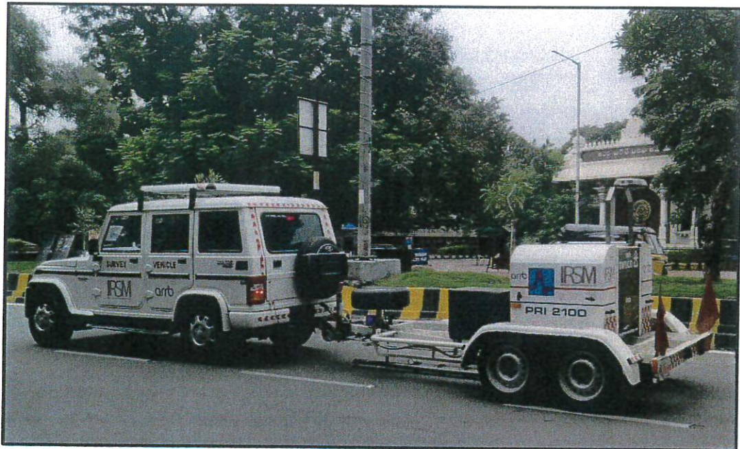
Photo 22: SWECO PRI 2100 FWD equipment
