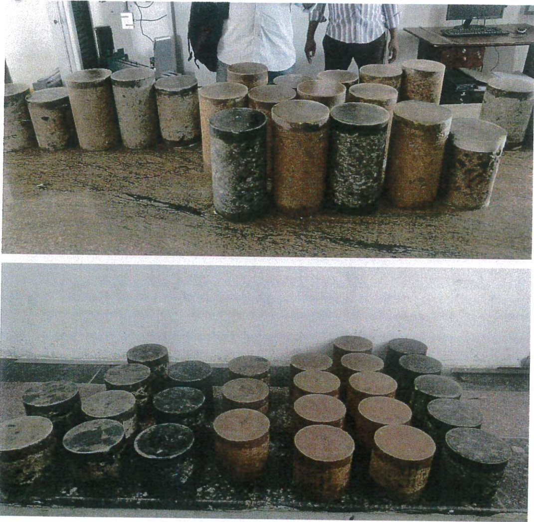
Photo 16 Field cores Trimmed and Levelled with Wax for UCS test
