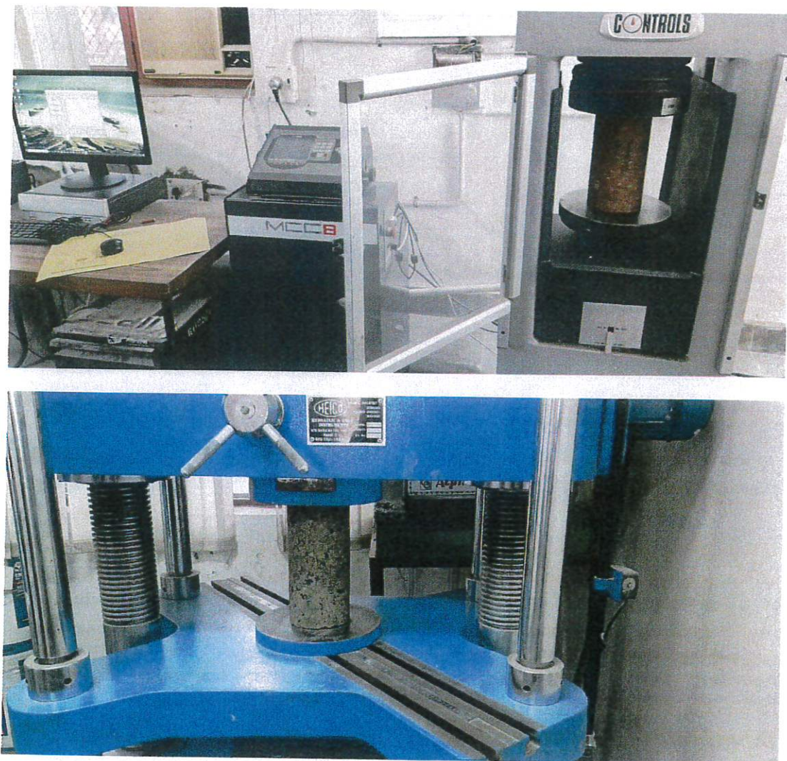
Photo 21 Residual UCS test (after durability cycles) on Stabilized cores
